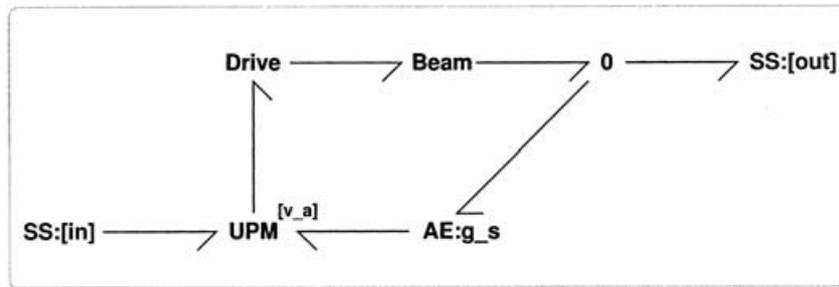
Fig. 12 Inner control loop bond graph
