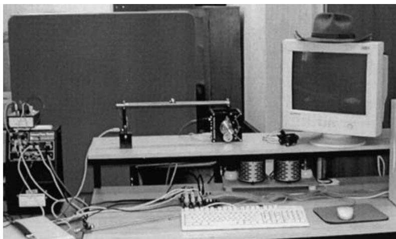
Fig. 7 Ball and beam apparatus
