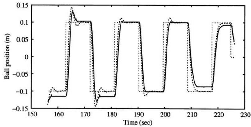
(a) Output, desired output and setpoint
