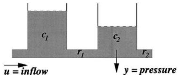
Fig. 4 Example: two coupled tanks
