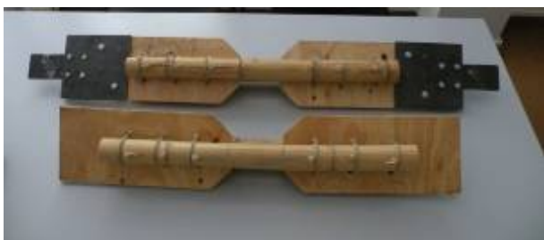
Figure 5. The specimen for traction tests on 3rd type joint.
