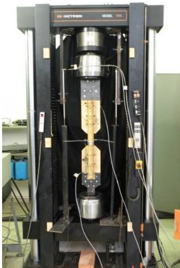
Figure 7. The traction tests on 3rd type joint.
