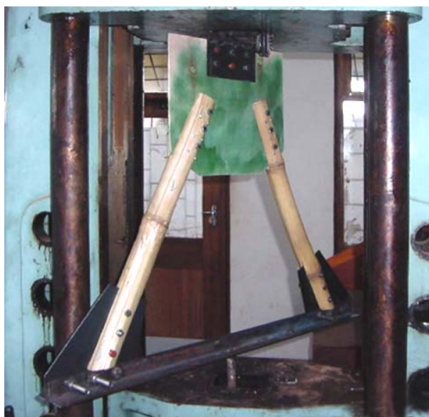
Figure 2. Tests on single and double 2nd type joints.
