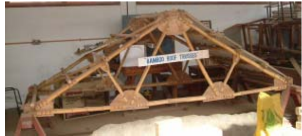
Figure 3. Truss with 2nd type joint.
