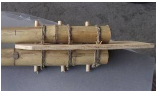
Figure 5. The specimen for traction tests on 3rd type joint.
