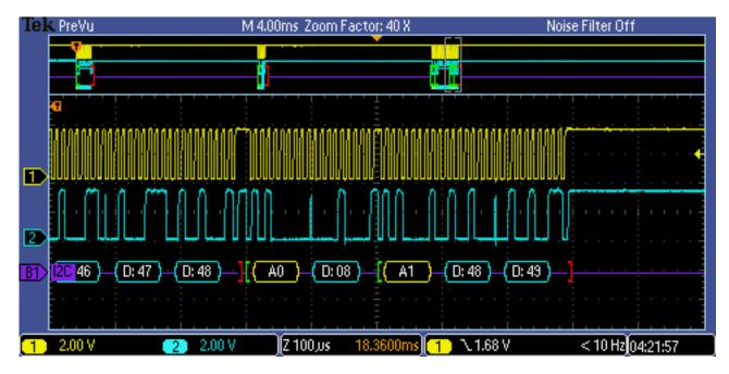
Figure 7: Last 2 bytes of 10 byte read
