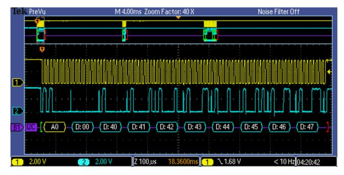
Figure 3: First section of a 10 byte write
