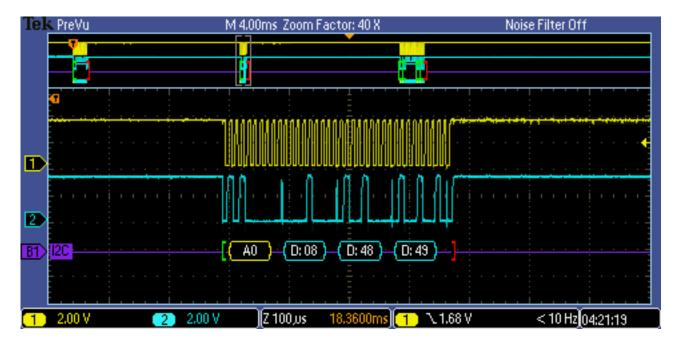
Figure 4: Second section of a 10 byte write
