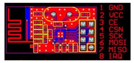
Figure 1: nRF24L01 Module
