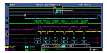
Figure 2: SPI I/O to nRF24
