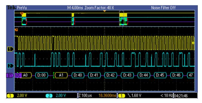
Figure 6: Eight byte burst read
