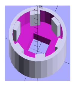
Figure 4: PTO Socket wrench
